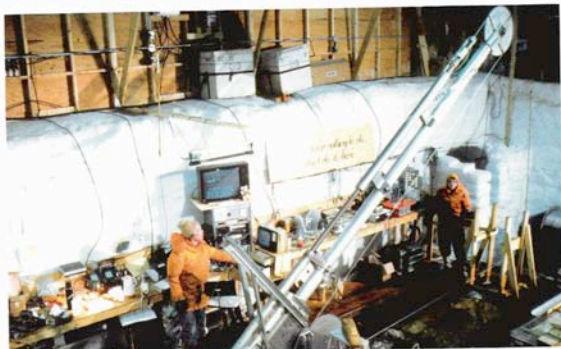
Fig. 10.2 The drill hall. ISTUK is being tilted by a hydraulic pump system.
